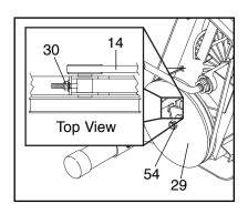
properly adjusted, reattach the side shields and pedals. If the Belt needs to be adjusted, loosen the Nylon Locknut (54) on the left side of the Flywheel (29). To tighten the Belt, turn the Adjustment Nut (30) clockwise; to loosen the Belt, turn the Adjustment Nut counterclockwise. Make sure that the Flywheel is straight and tighten the Nylon Locknut (54). Reattach the side shields and pedals.
